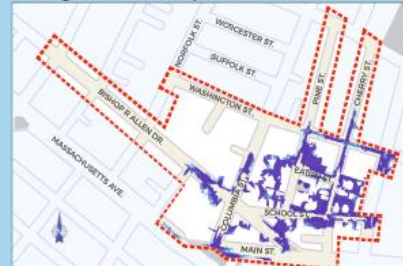
Anticipated flooding for a 2030, 10 year / 24 hour storm
