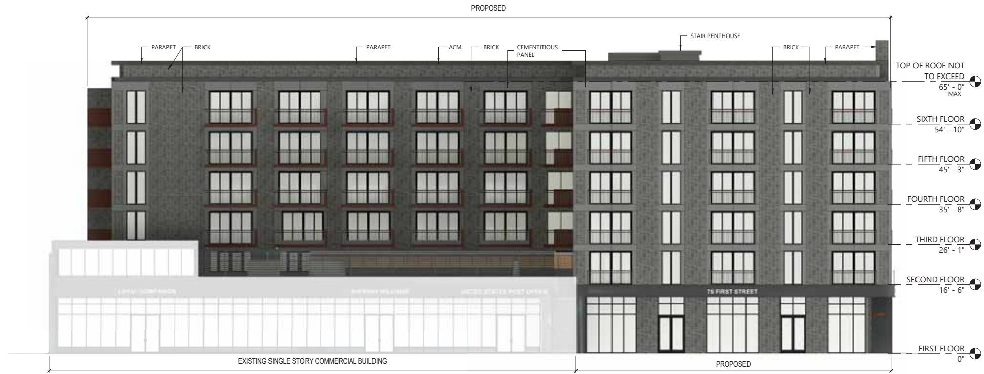
1 FIRST ST ELEVATION (LOOKING WEST) 3/32" = 1'-0"
