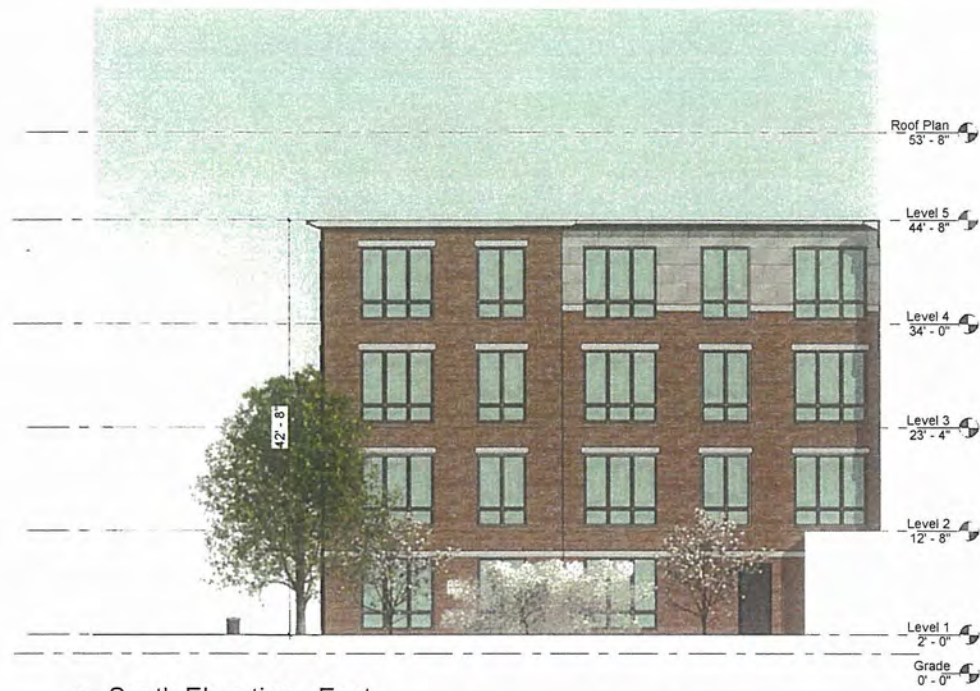
3 South Elevation - East 1/8" = 1'-0"
