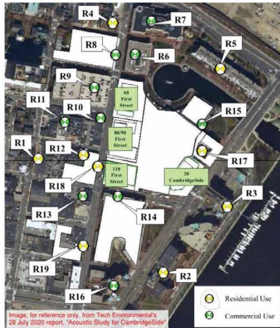
Figure 10 – Noise-Sensitive Receiver Locations Evaluated for Tech Environmental's Assessment of CambridgeSide Redevelopment Project Rooftop Noise Emissions
