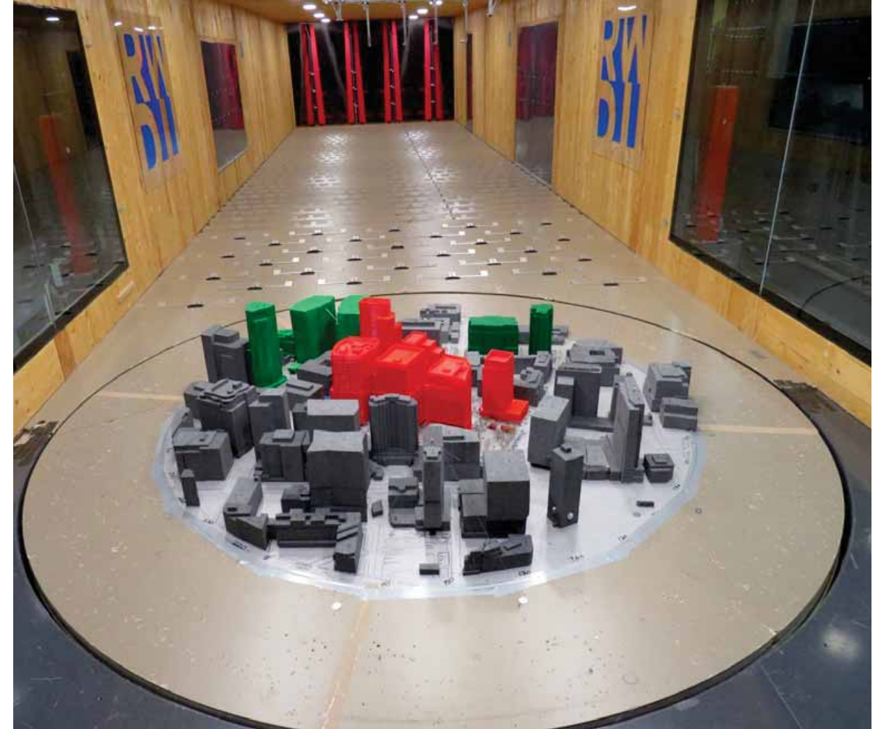
Image 2F: Wind Tunnel Study Model – Full Build
