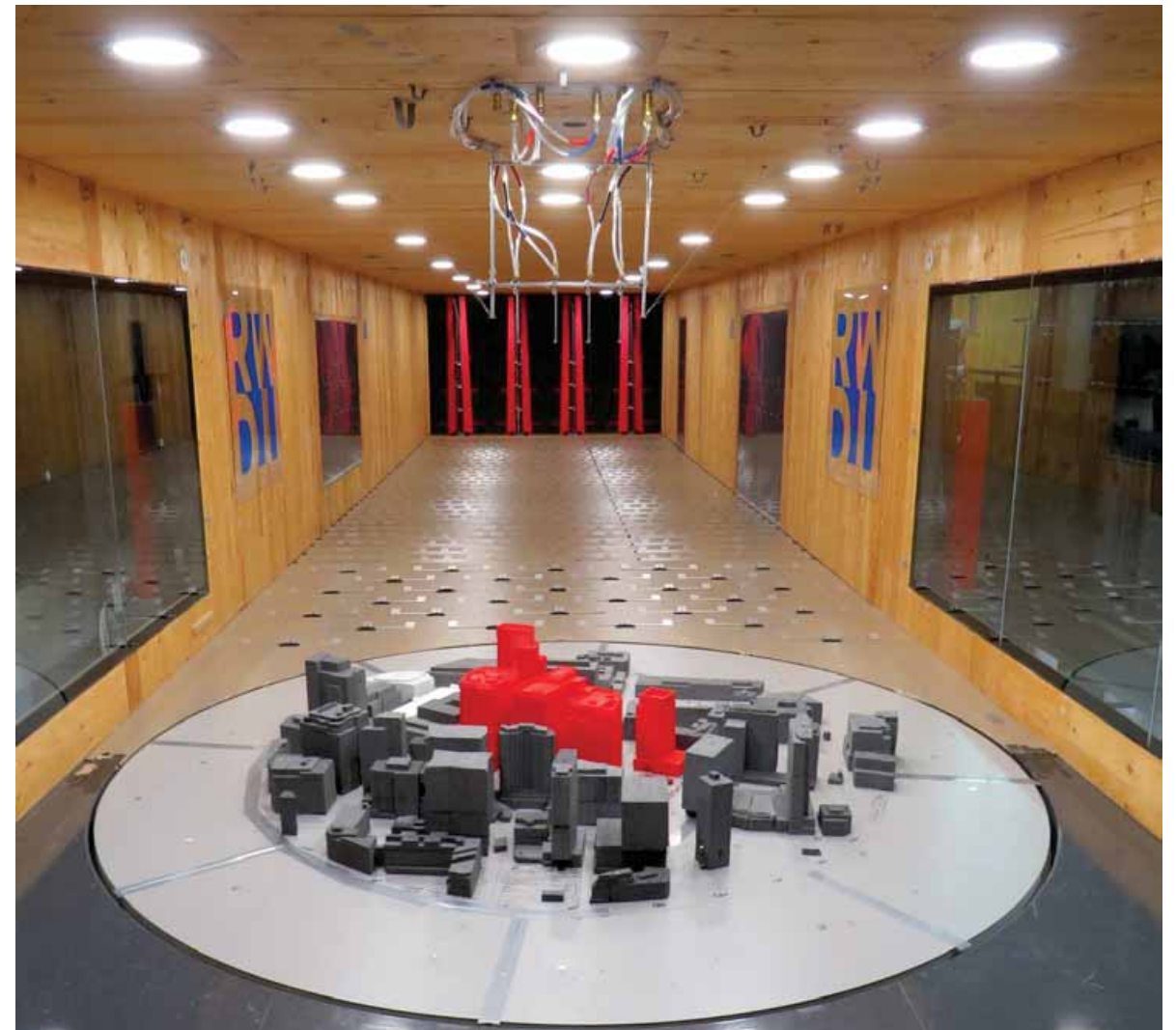
Image 2D: Wind Tunnel Study Model – Build
