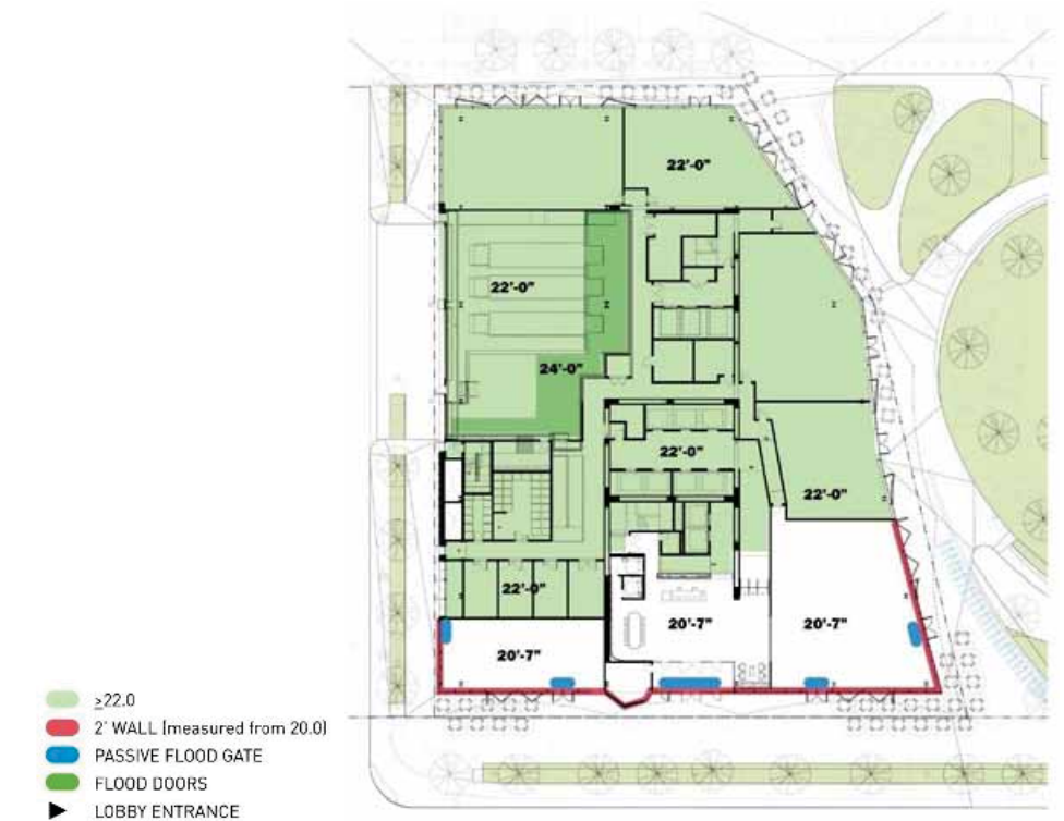
Figure 9 - Volpe Site Flood Mitigation Strategies
