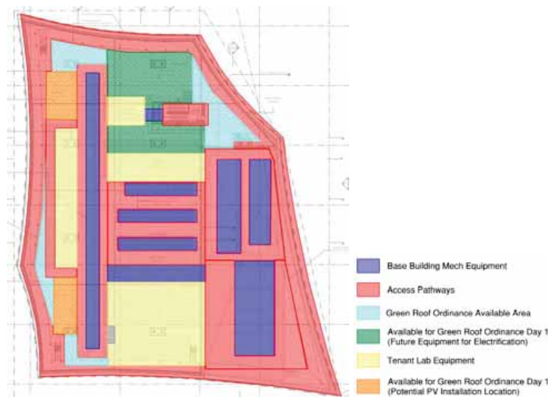
Figure 8 – C1 Roof Area
