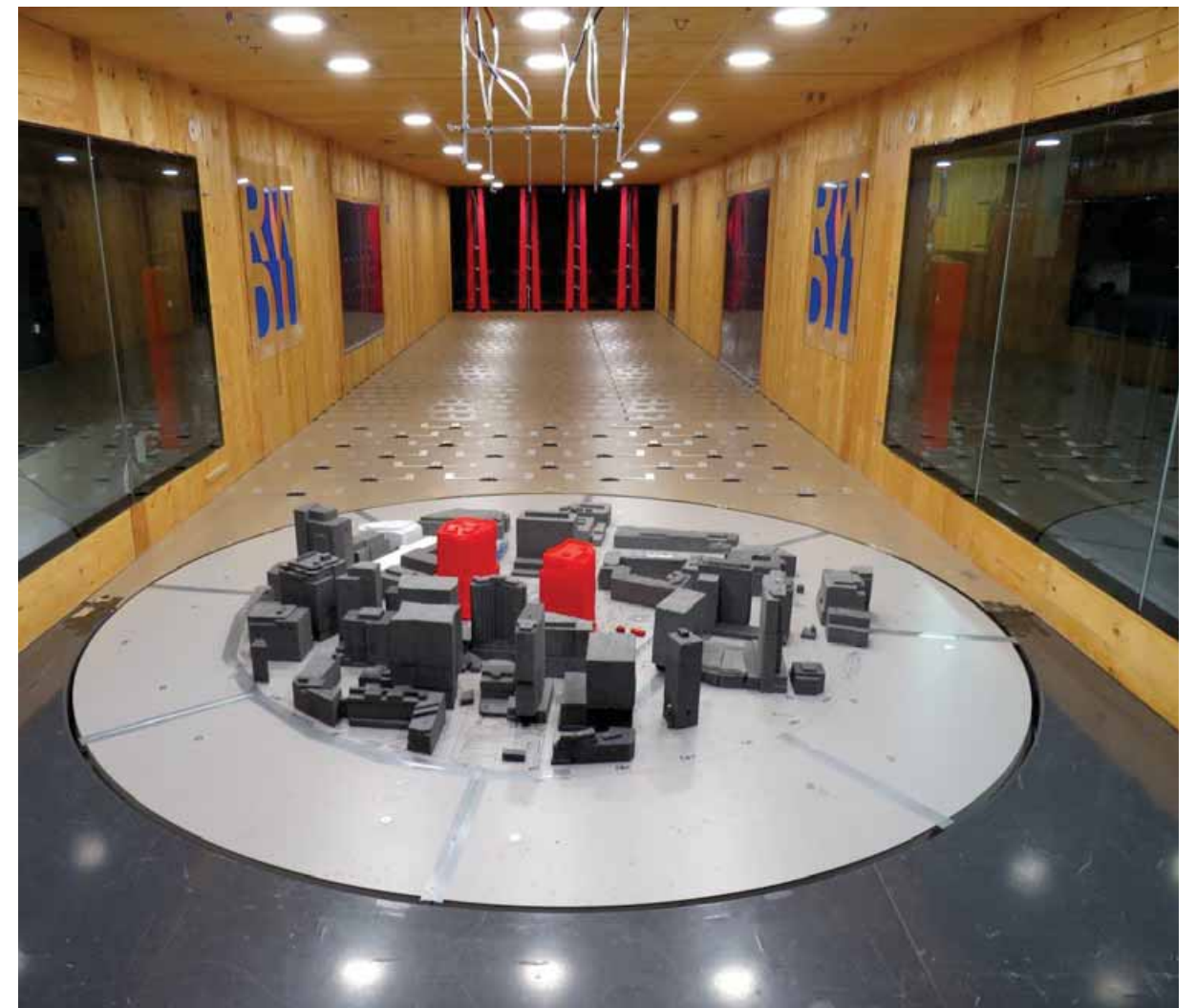
Image 2B: Wind Tunnel Study Model – Build C1 & C3
