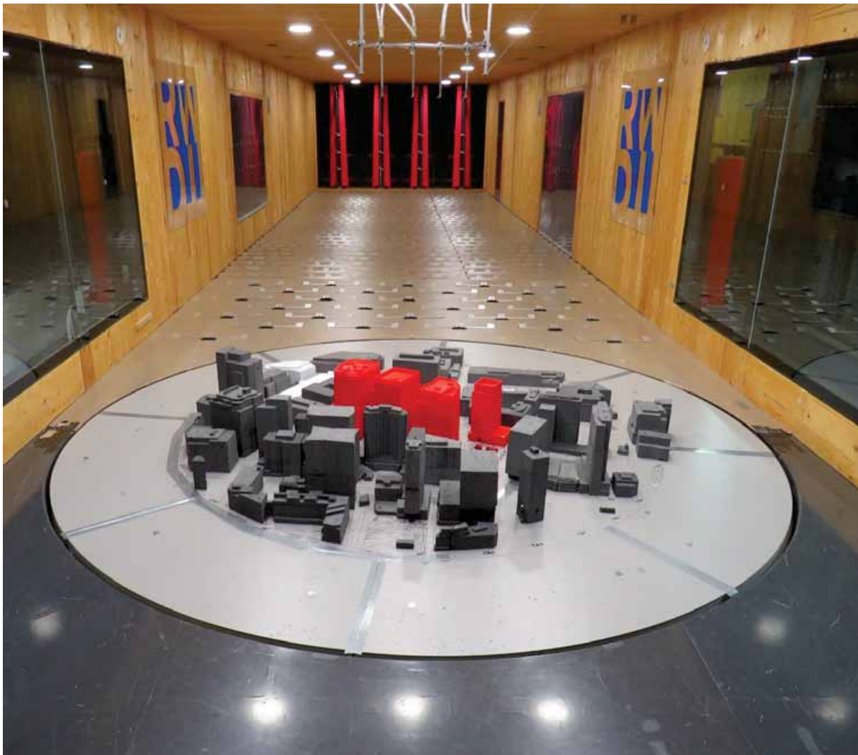
Image 2C: Wind Tunnel Study Model – Build C1, C2, C3 & R1
