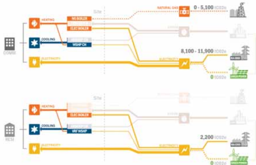
Figure 10. Potential Electric-ready Commercial and All-electric Residential Pathway, Pending Grid Reliability. Grid emissions projected at current level but expected to decrease over time. To be further evaluated when buildings enter design.
