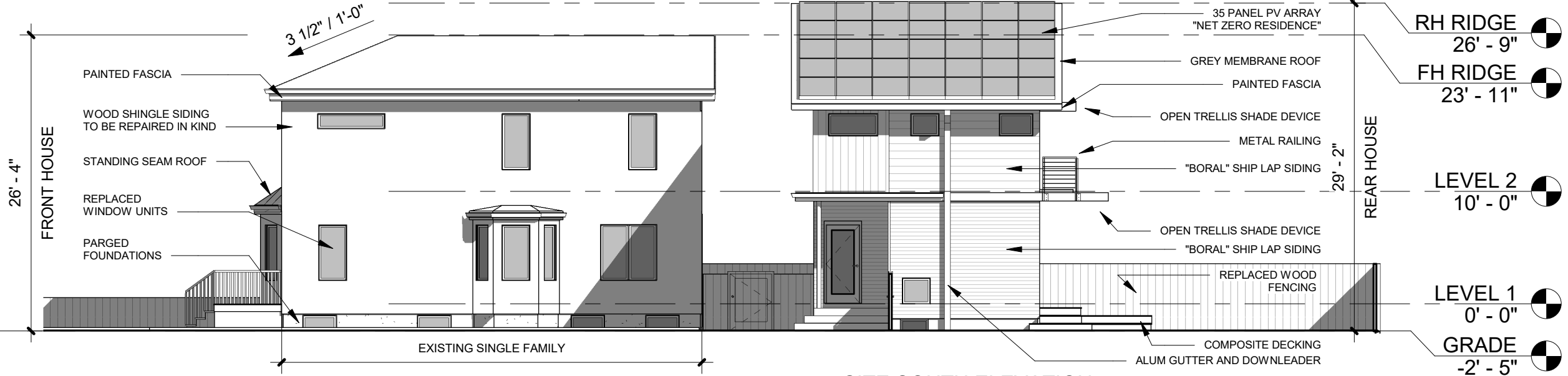
01 SITE SOUTH ELEVATION 3/32" = 1'-0"
