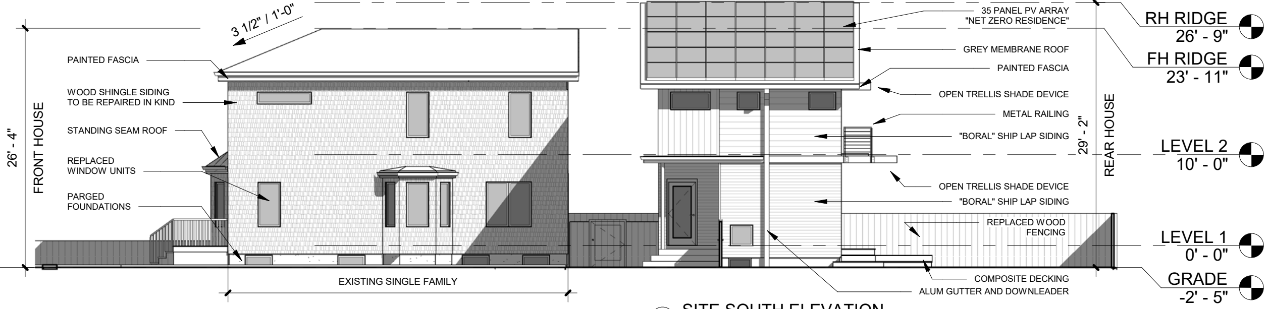
01 SITE SOUTH ELEVATION 3/32" = 1'-0"
