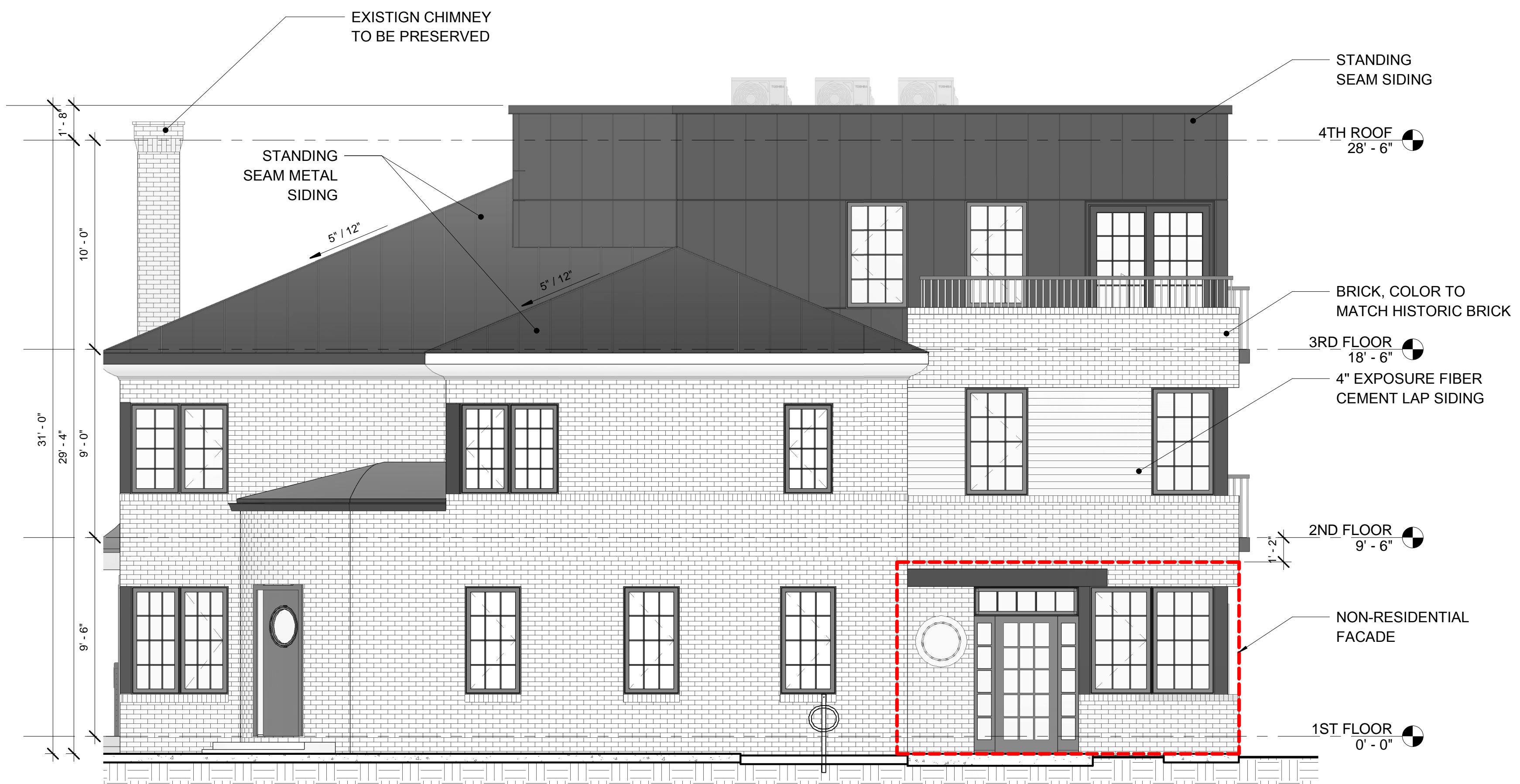
1 SOUTH WEST ELEVATION 1/4" = 1'-0"
