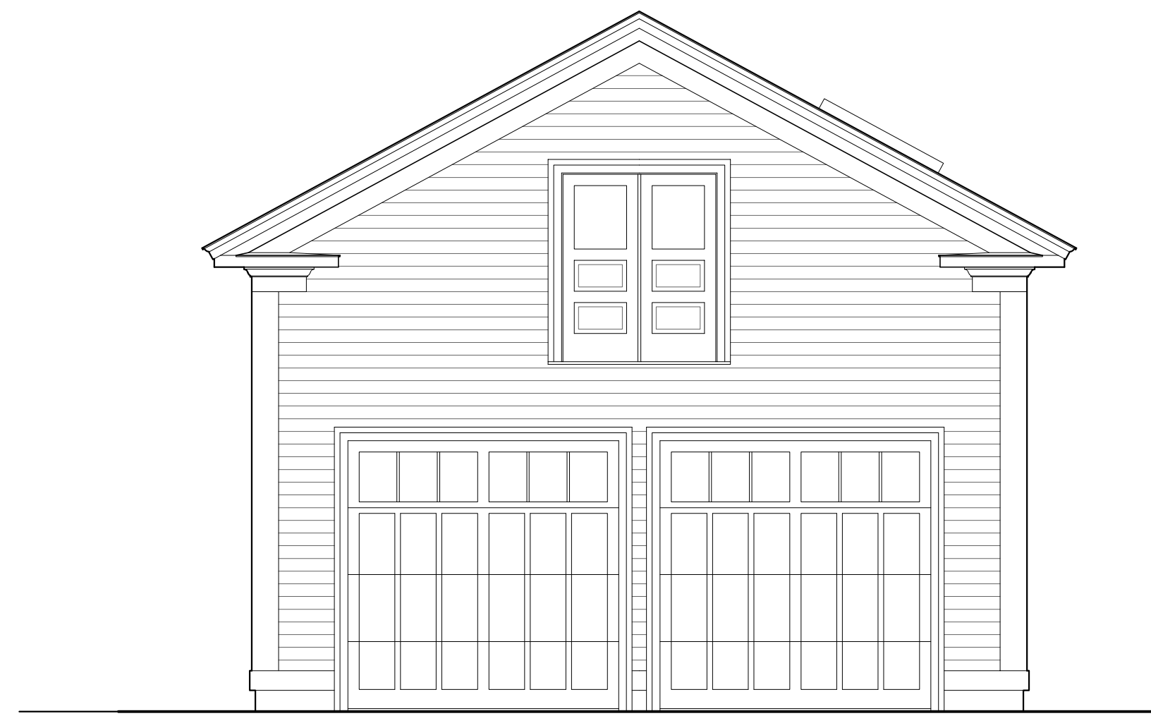
3 CARRIAGE HOUSE EAST ELEVATION SCALE: 1/4" = 1'-0"
