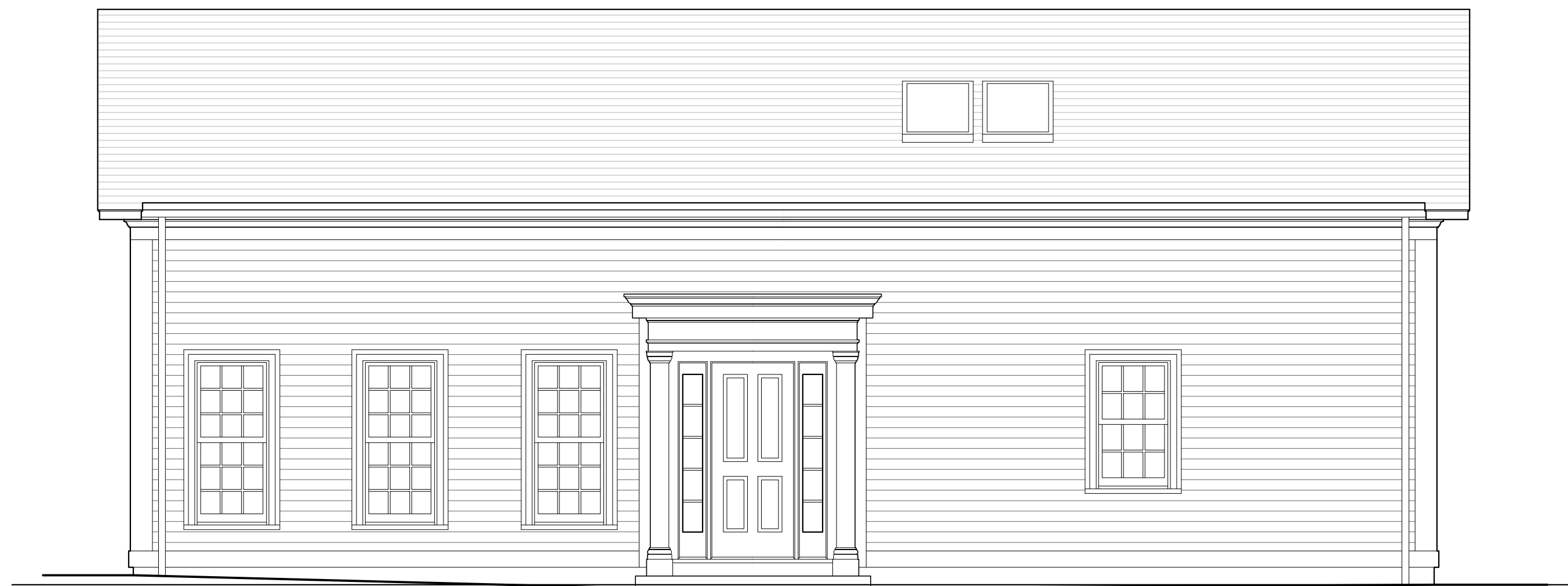
5 CARRIAGE HOUSE SOUTH ELEVATION SCALE: 1/4" = 1'-0"
