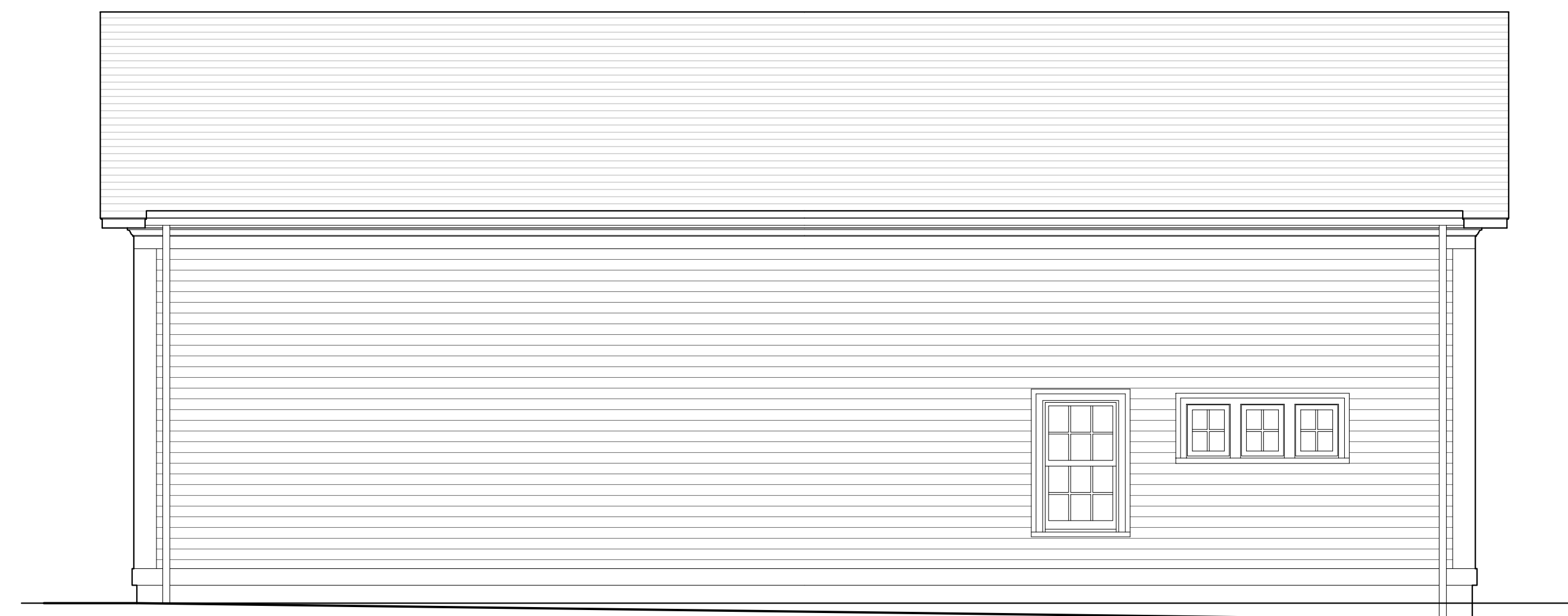
6 CARRIAGE HOUSE NORTH ELEVATION SCALE: 1/4" = 1'-0"
