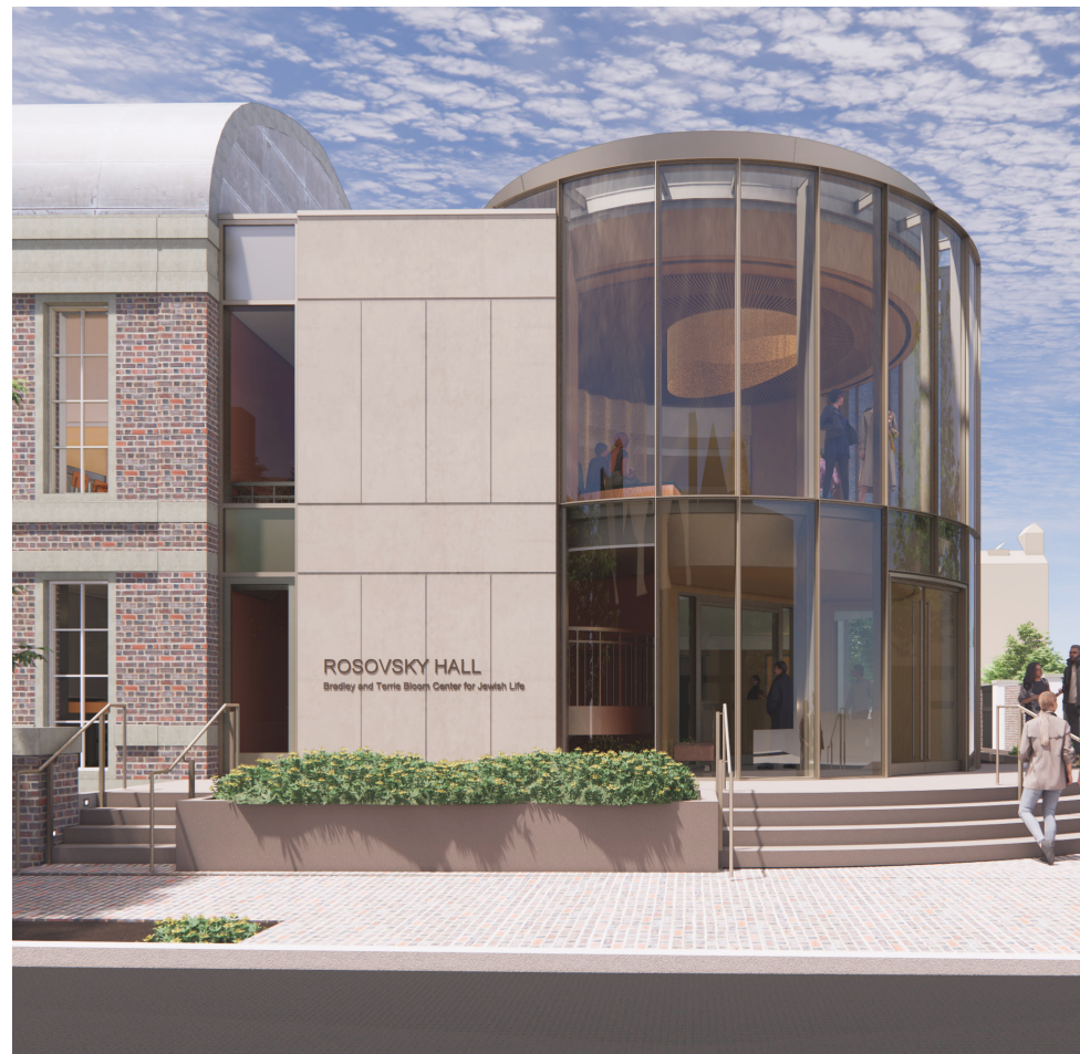
ENTRY PAVILION (CAST STONE PANEL WALL, METAL AND GLASS CURTAINWALL)
