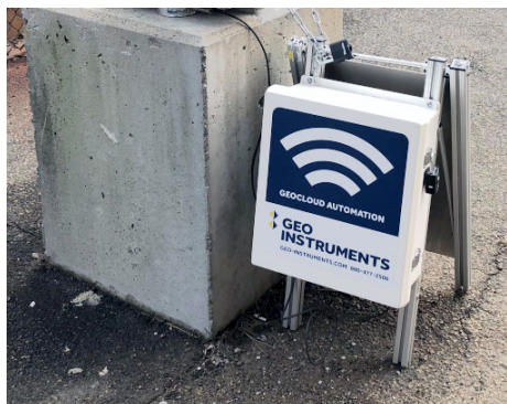
Typical vibration monitoring equipment.
