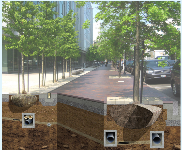
Main Street in Kendall Square demonstrates the system of soil and drainage necessary for healthy street trees to grow and thrive.
