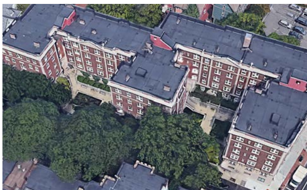
Large developments should include semi-public forecourts to break up long building facades.
