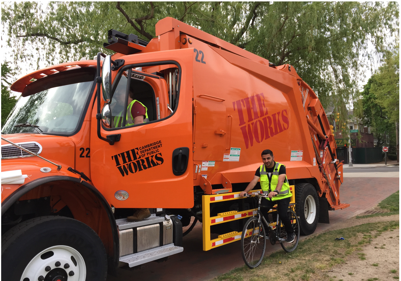
Figure 3.20: Cambridge Department of Public Works employees demonstrating truck side guards on City trucks.
