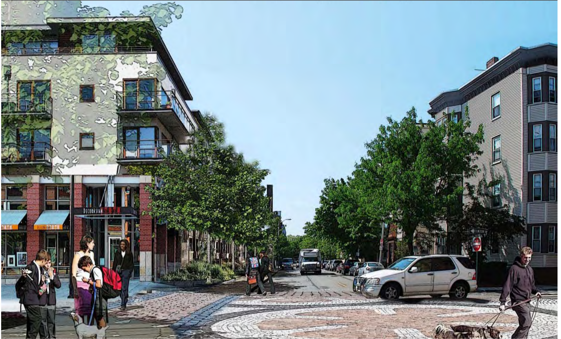
45' façade height limit at Bishop Allen. 45 degree height limit plane tapers back above.
