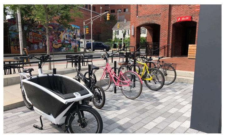
Figure 7.2: Bike rack designs need to accommodate the diversity of bike shapes and sizes, including cargo bikes and adaptive bikes.
