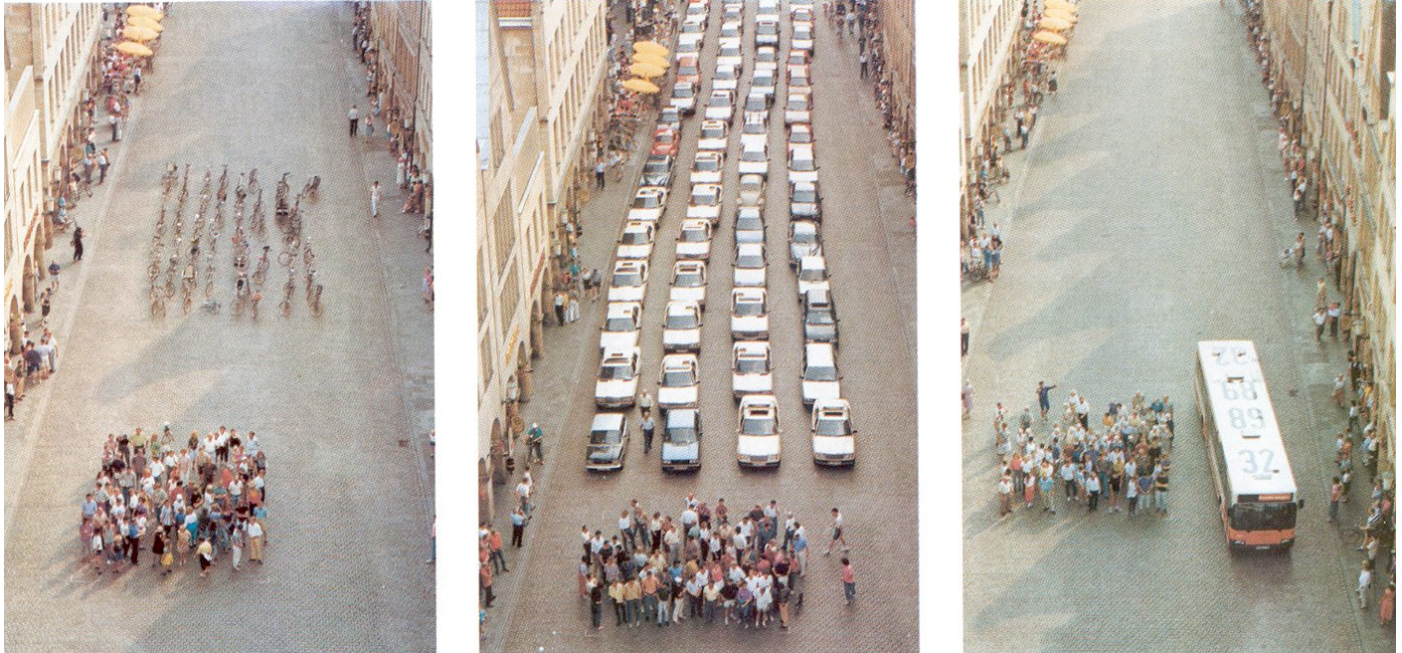
Figure 2.2: Relative space for different travel modes. In this influential photo, the City of Münster, Germany demonstrates the relative space required to move the same number of people by bicycle, car and bus. 7
