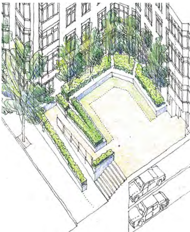
Elevated forecourt, with steps and ramps up from sidewalk level, giving access to the building's elevated lobby. .
