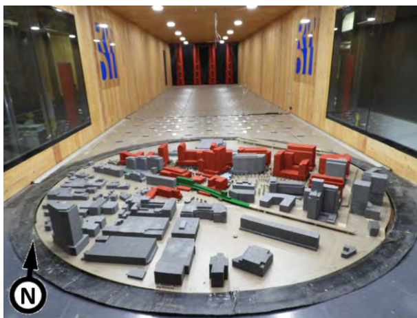
Image 2: Wind tunnel study model - proposed configuration
