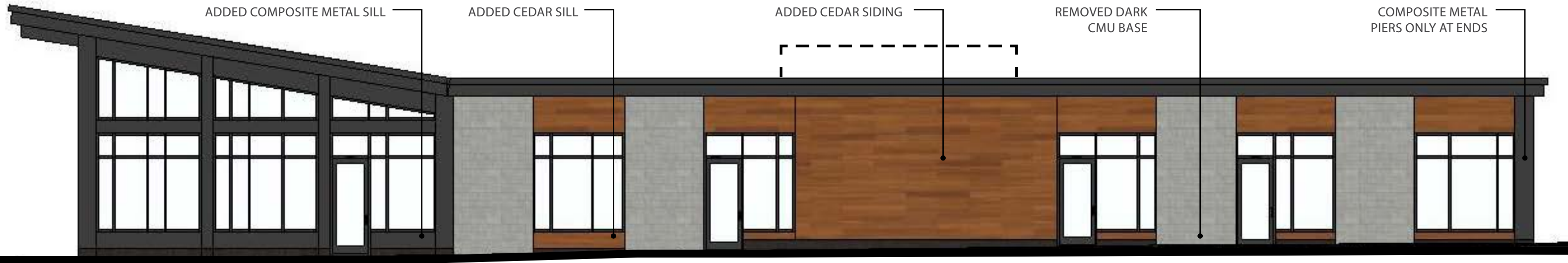
PROPOSED 2021 EAST BUILDING NORTH ELEVATION
