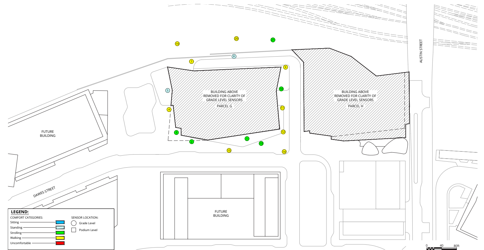
Pedestrian Wind Comfort Conditions Future Configuration Winter (November to April, 6:00 to 23:00) Parcel G & H - Northpoint Site - Cambridge, MA True North Drawn by: DBB Figure: 2 Approx. Scale: 1"=80' Project #1703124 Date Revised: Sept. 26, 2017
