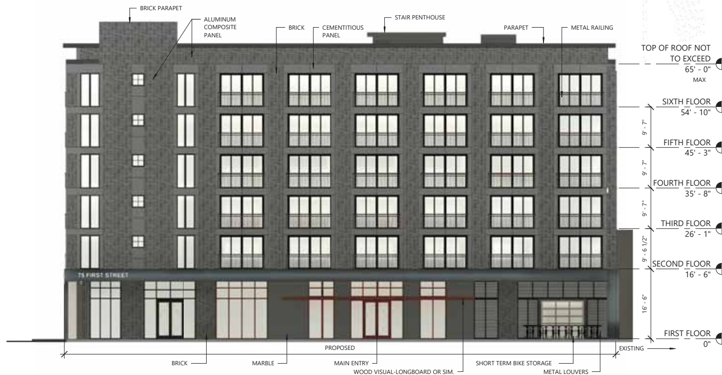
2 SPRING ST ELEVATION (LOOKING SOUTH) 3/32" = 1'-0"
