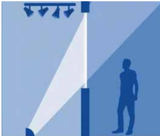
Light reflective glazing solutions and light reducing filming to reduce interior light casting out
