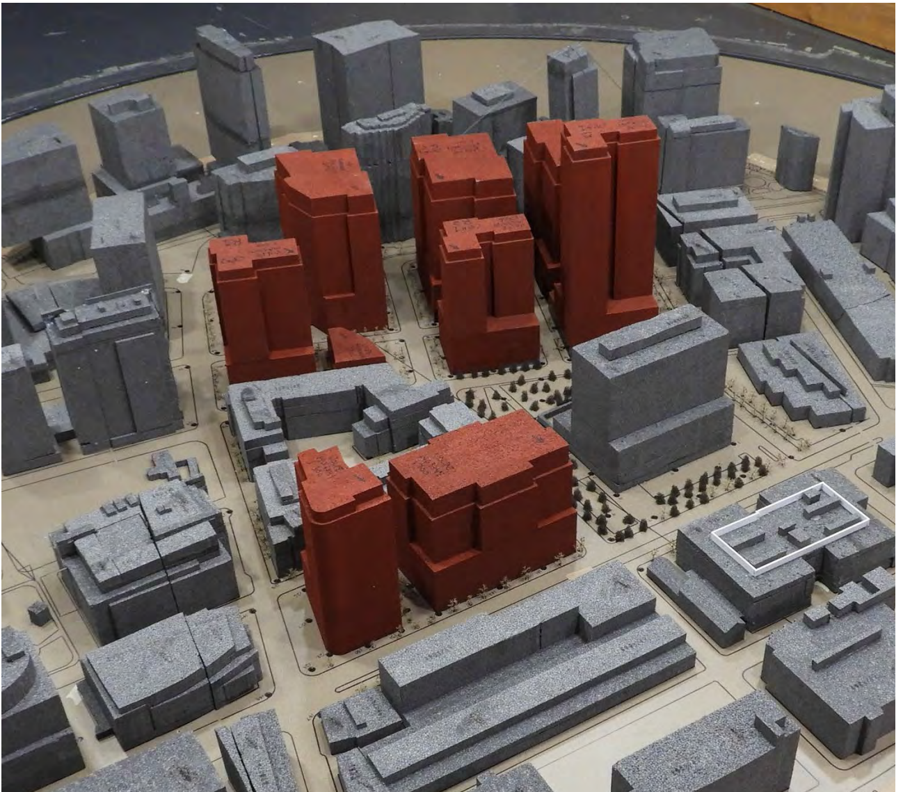
Image 2B: Wind Tunnel Study Model – Build Configuration
