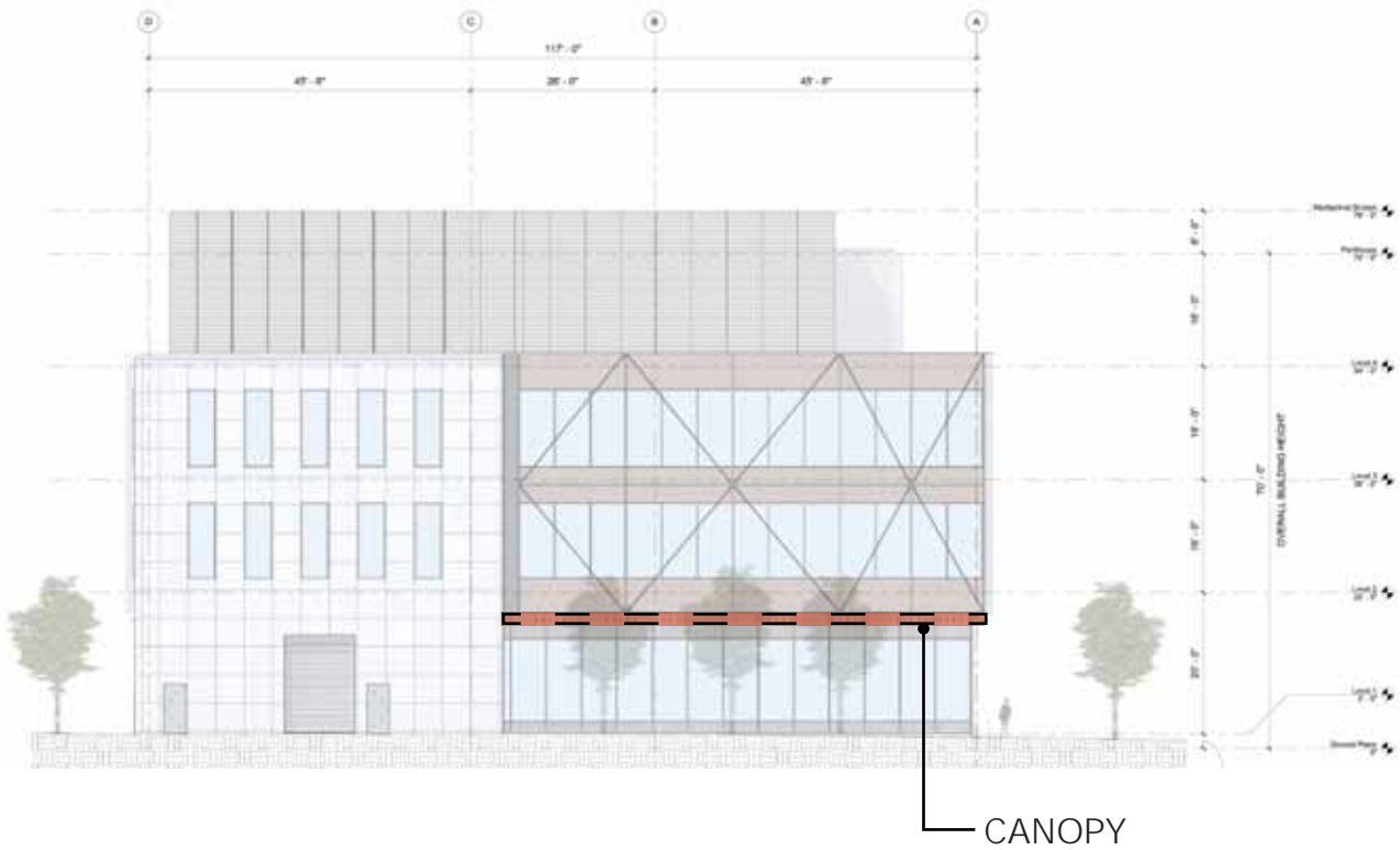
CANOPIES AND TENANT ENTRANCES - NORTH ELEVATION
