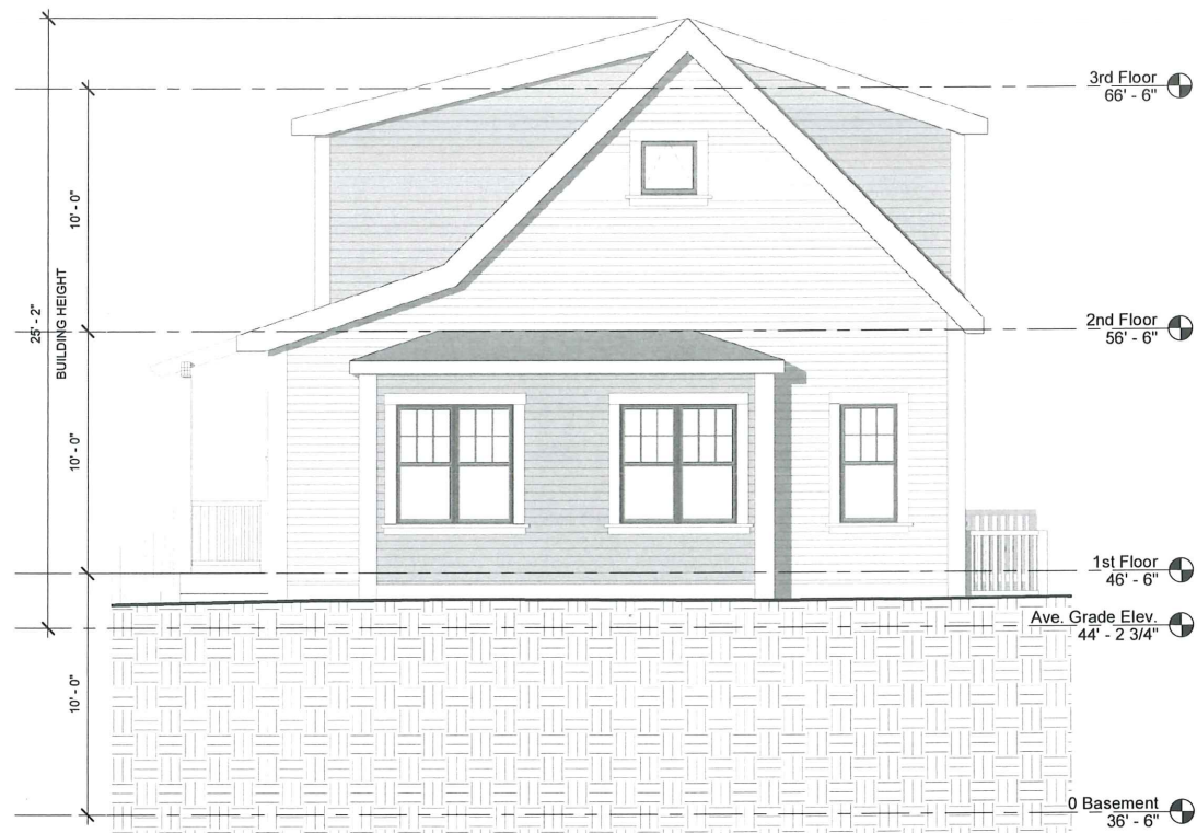
③ South Elevation - Front Unit 1/4" = 1'-0"
