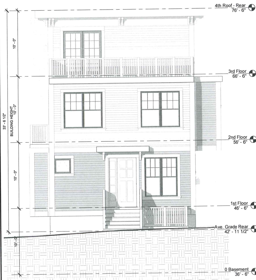
④ West Elevation - Rear Unit 1/4" = 1'-0"
