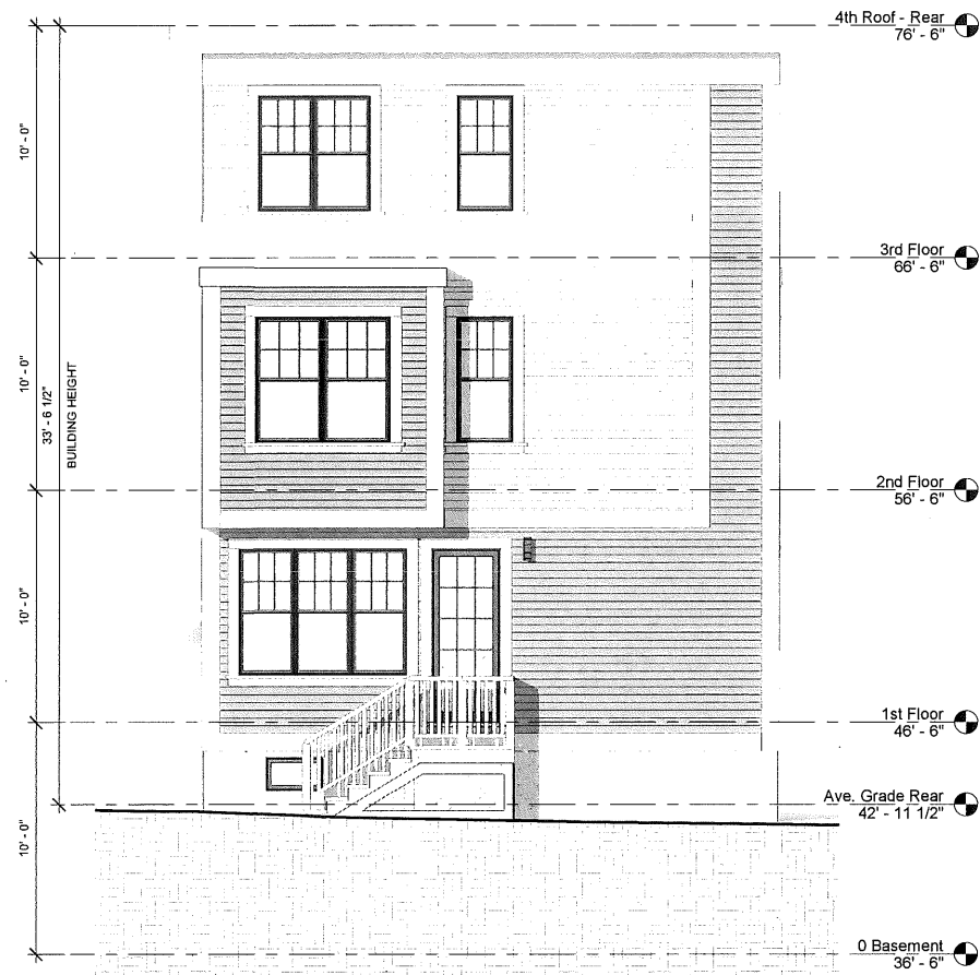
① East Elevation - Rear Unit 1/4" = 1'-0"
