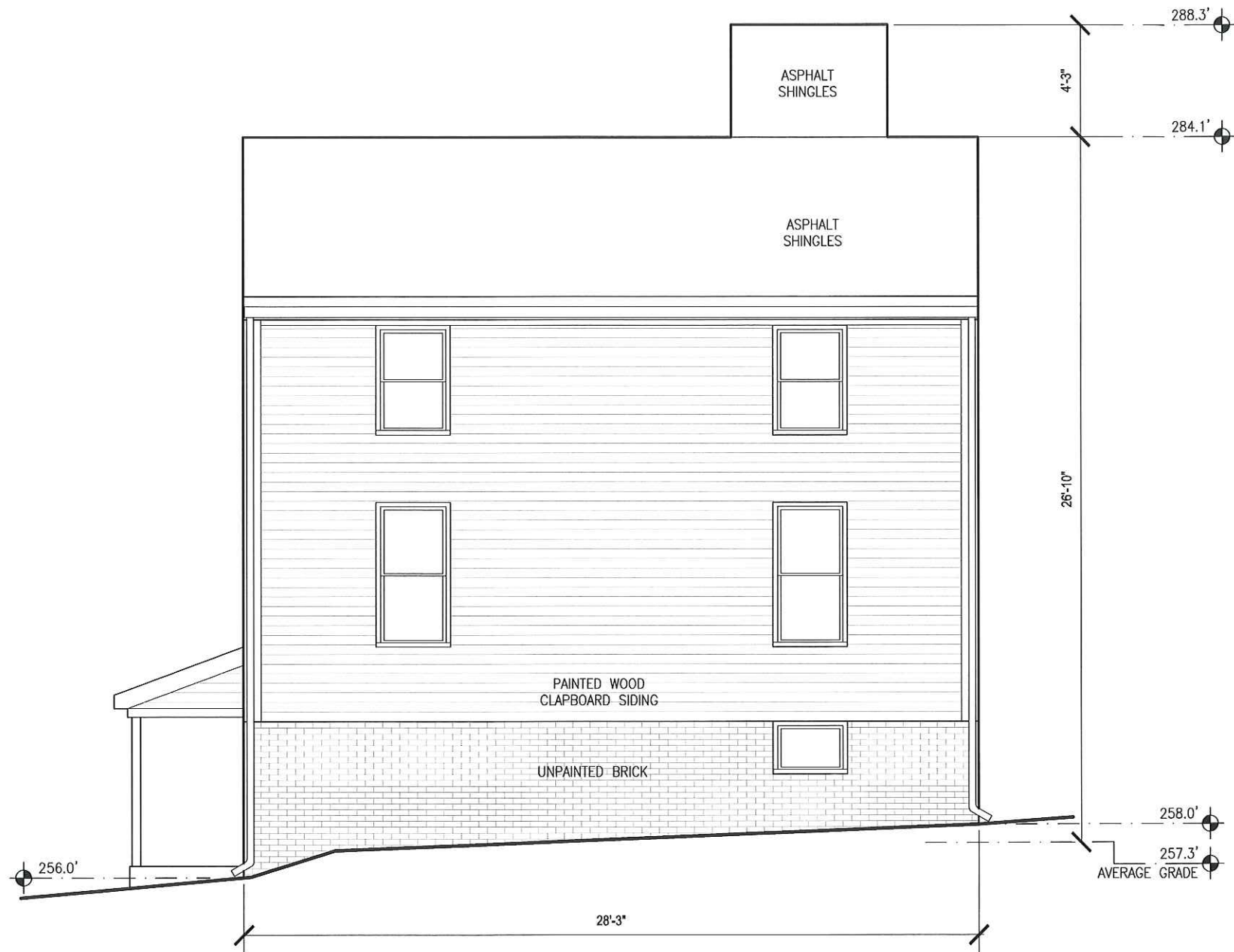
1 EXISTING ELEVATION - NORTH SCALE: 3/16" = 1'
