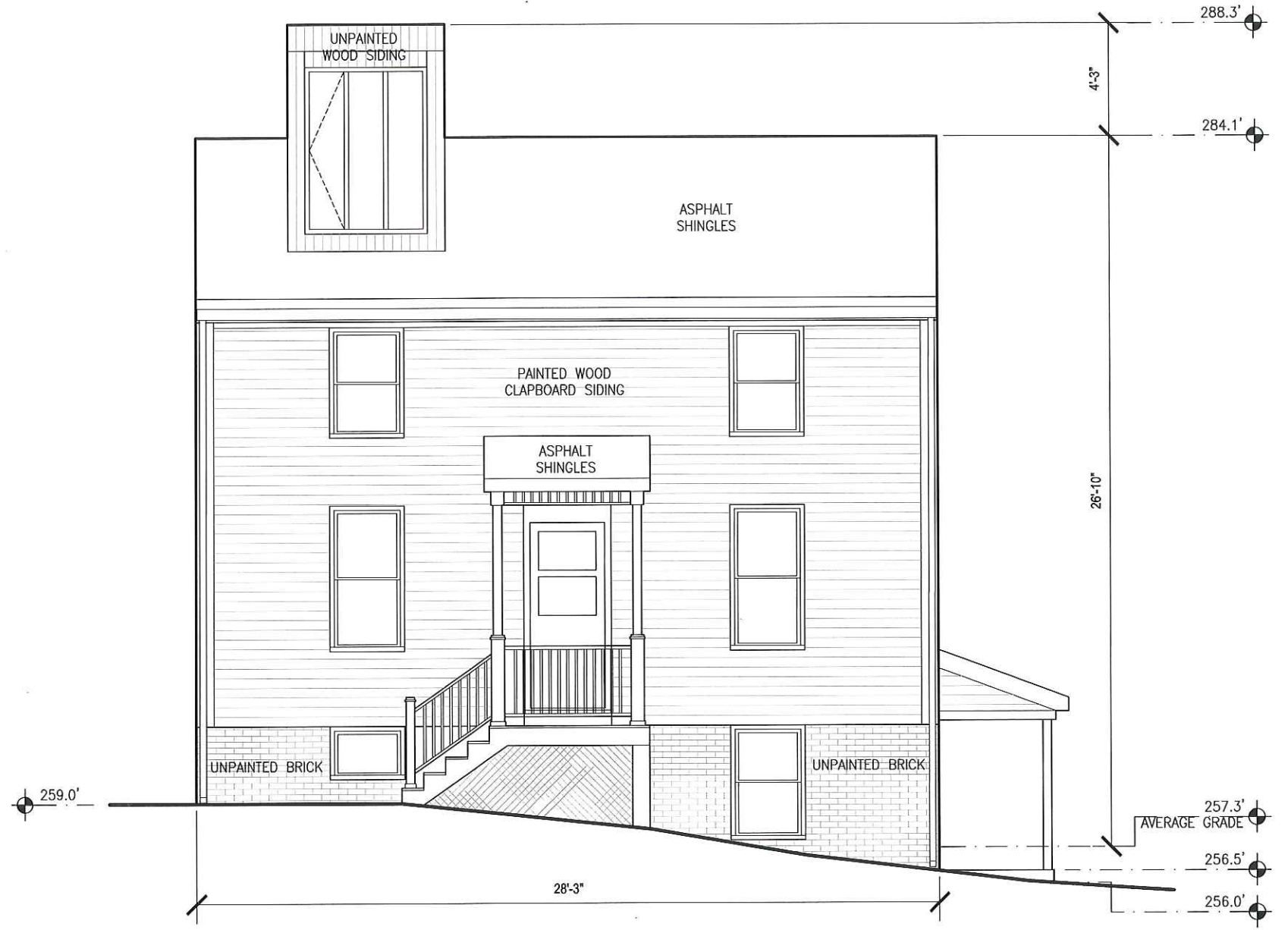
2 EXISTING ELEVATION - SOUTH SCALE: 3/16" = 1'
