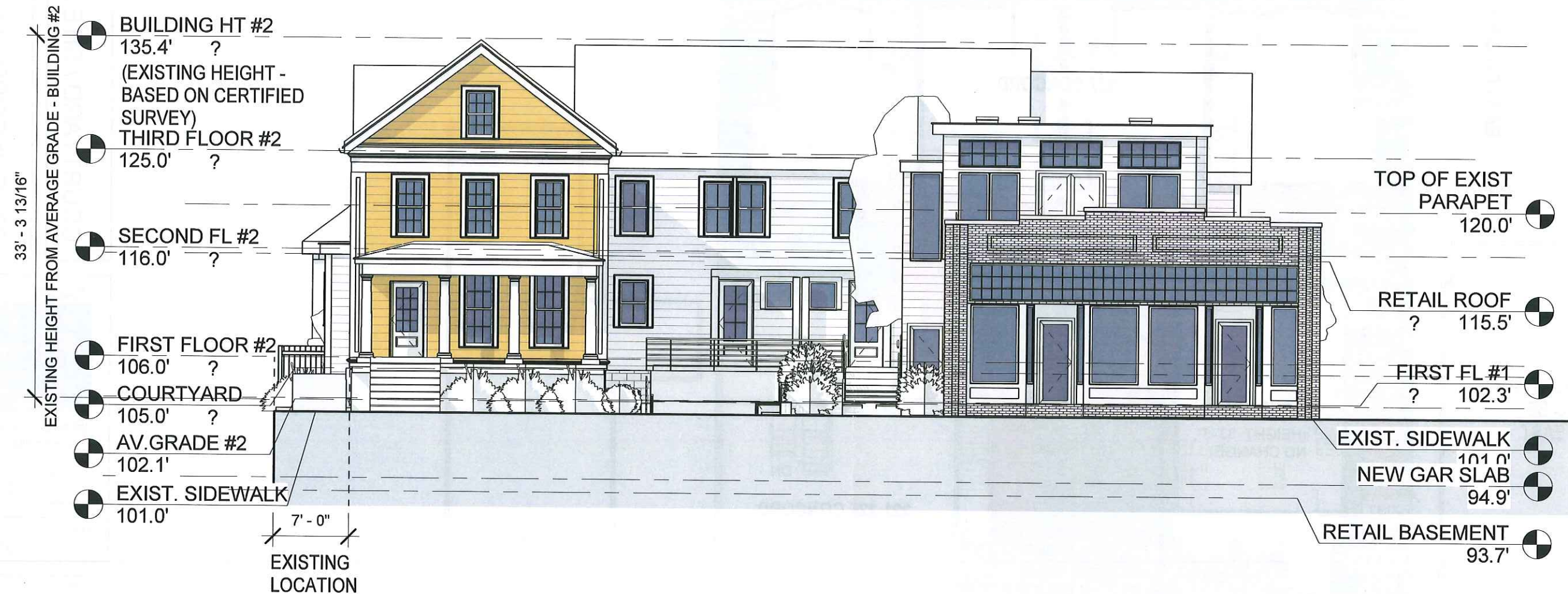
1 SOUTH / FRONT OVERALL SITE ELEVATION - AS PERMITTED 3/32" = 1'-0"
