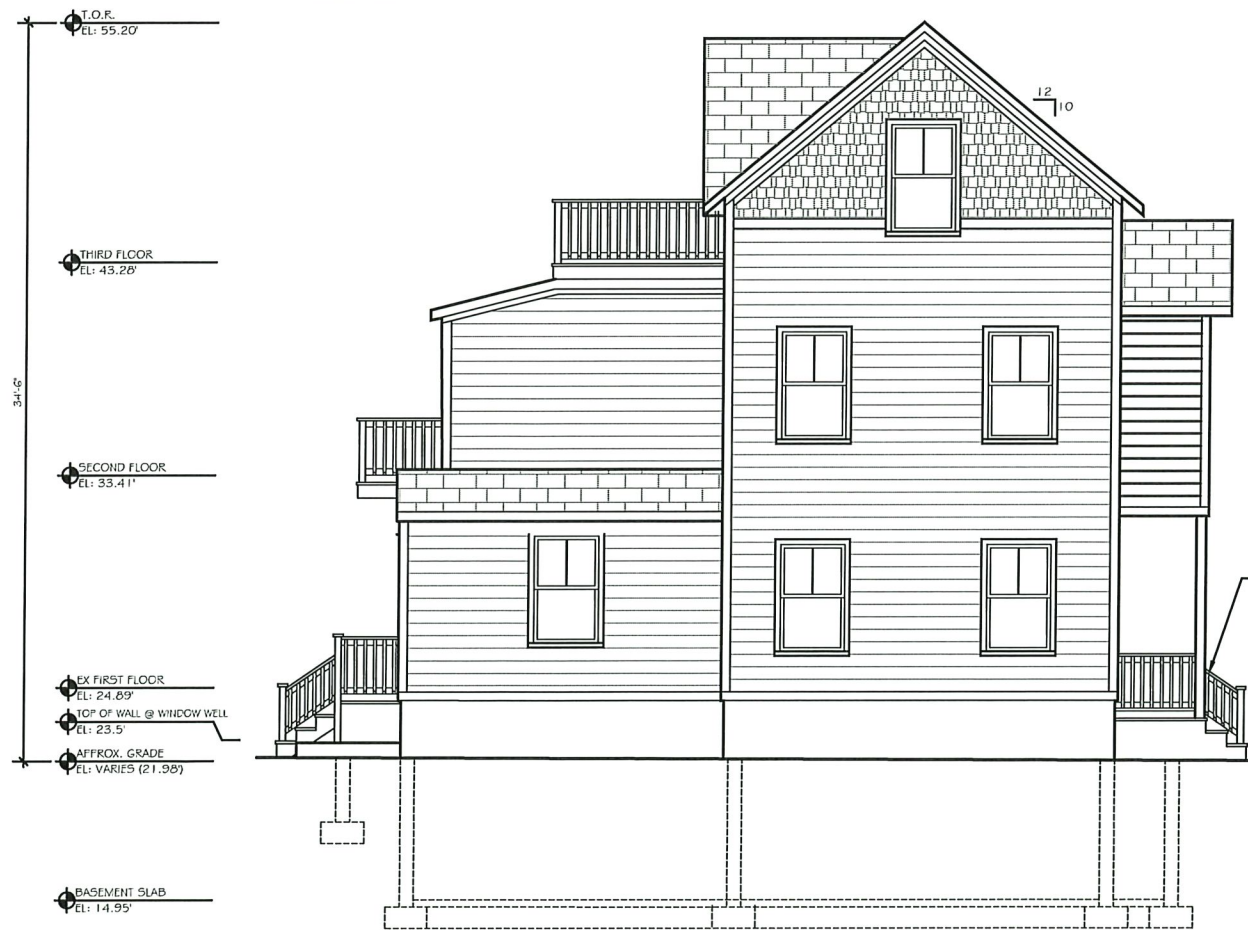
PROPOSED LEFT SIDE ELEVATION SCALE 1/4" = 1'-0"
