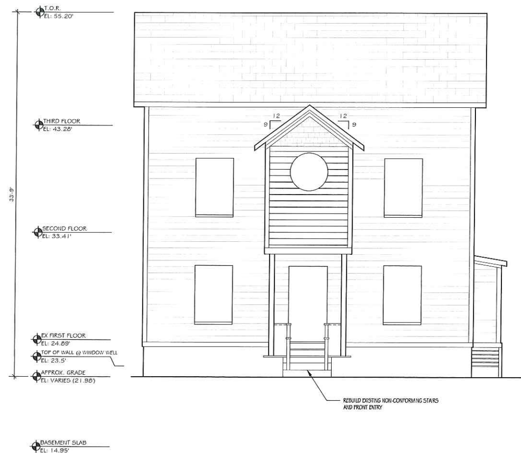
PROPOSED FRONT ELEVATION SCALE 1/4" = 1'-0"
