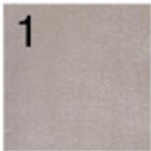
1 No aggregate Typical sidewalk concrete Smooth
