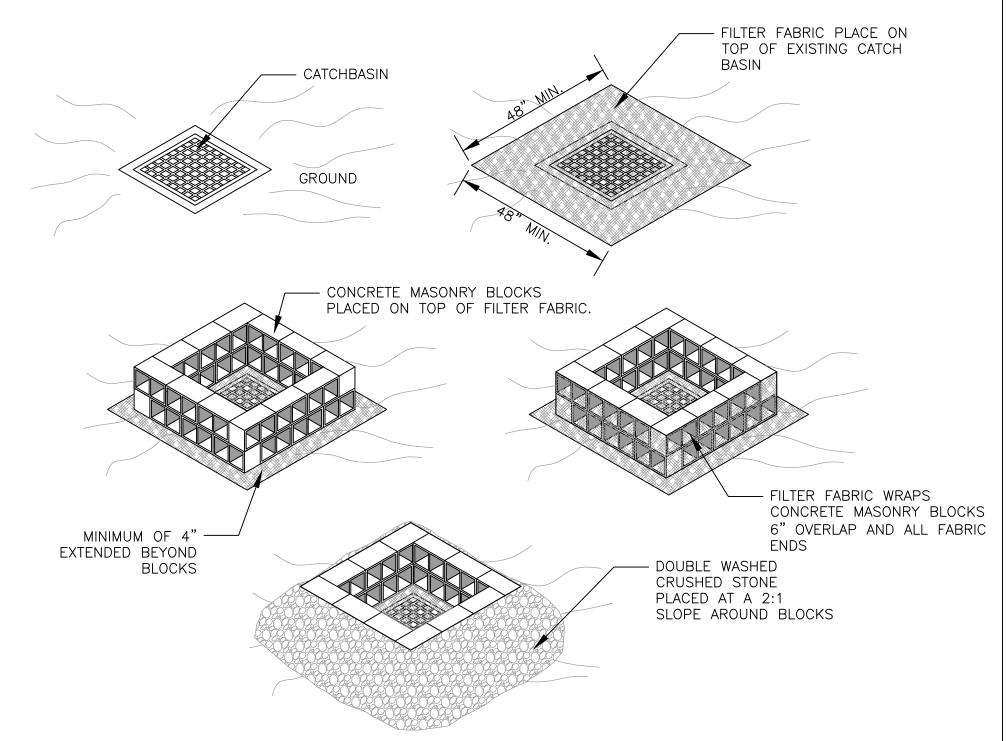
THIS METHOD OF INLET PROTECTION IS APPLICABLE WHERE HEAVY FLOWS ARE ANTICIPATED AND OVERFLOW CAPACITY IS NECESSARY TO PREVENT EXCESSIVE PONDING
