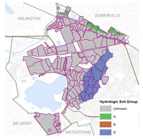
Figure 6. Hydrologic Soil Group (HSG) Classification in the Alewife Area
