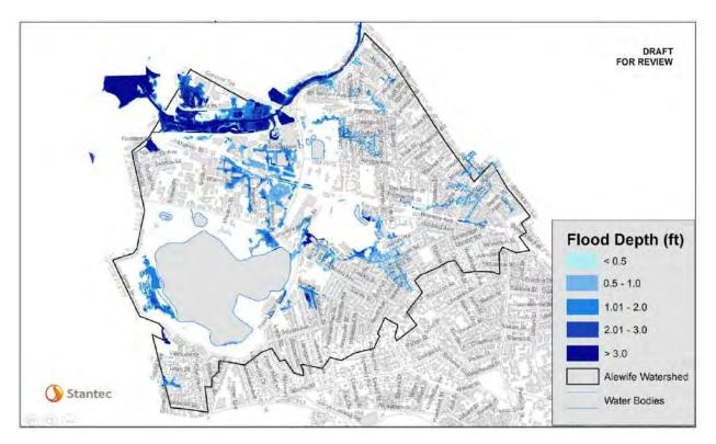
Figure 4a. Flood Depth with Current Infrastructure Conditions, 10-year 24hr Storm, 2070 using 3 Pumps at the Amelia Earhart Dam, Cradock Locks Removed (InfoWorks ICM Integrated Model)
