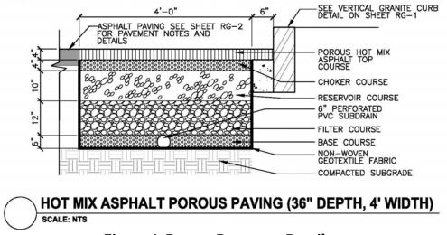
**Figure 4: Porous Pavement Detail**
