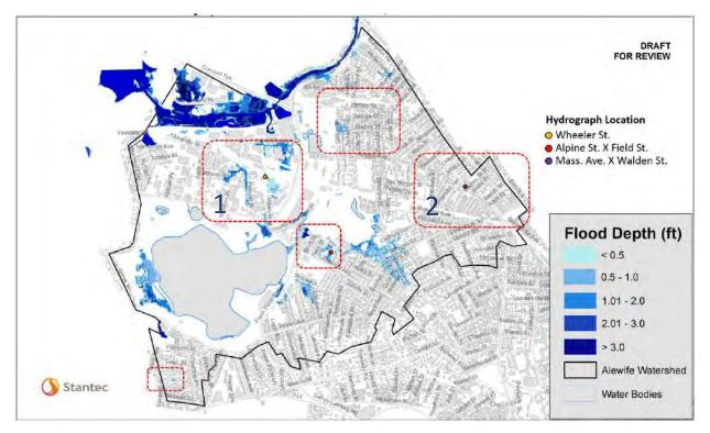
Figure 4b. Flood Depth with Green Infrastructure at MEP, 10-year 24hr Storm, 2070 using 3 Pumps at the Amelia Earhart Dam, Cradock Locks Removed (InfoWorks ICM Integrated Model)
