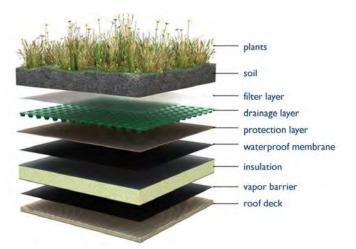
**Figure 9: Typical Extensive Green Roof Section**
