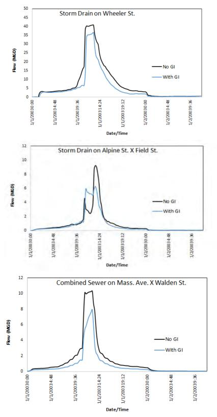
Figure 3. Flow hydrographs for the 10-year, 24-hour under 2070 horizon with and without GI implementation in Alewife.
