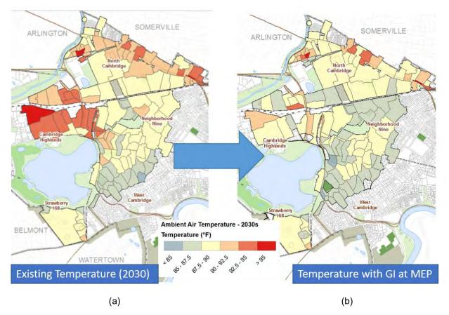
Figure 13. 2030 mean ambient air temperature summarized at the subcatchment scale under (a) existing conditions with no green infrastructure, and (b) proposed conditions with green infrastructure
