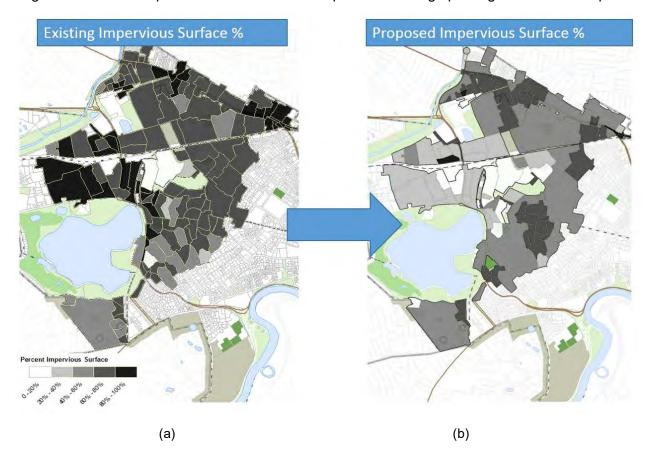
Figure 12. Percent imperviousness summarized at the subcatchment scale under (a) existing conditions with no green infrastructure, and (b) proposed conditions with green infrastructure
