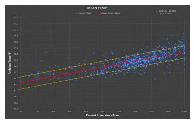
Figure 11: Relationship between ambient air temperature and percent imperviousness under existing conditions
