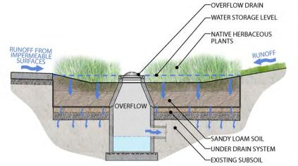
**Figure 2: Bioretention Basin Typical Section**
