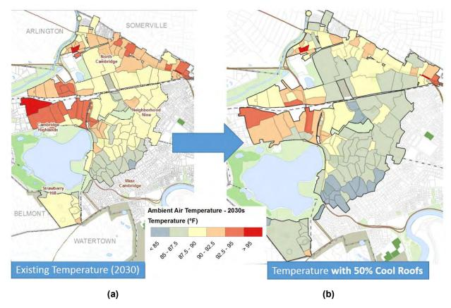
Figure 21: 2030 Mean Ambient Air Temperature Summarized at the Subcatchment Scale under (a) Existing Conditions, and (b) Proposed Conditions with 50% Implementation of White Roofs
