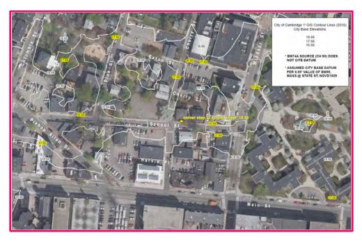
Figure 8: High water elevation from July 10, 2010 flood on School St (Source: City of Cambridge)<sup>11</sup>
