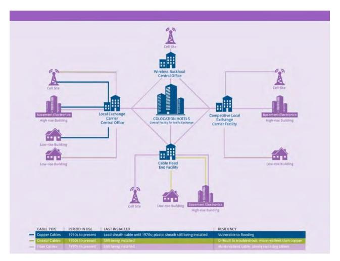
Figure 1: Diagram of Telecommunications Components<sup>98</sup>.
