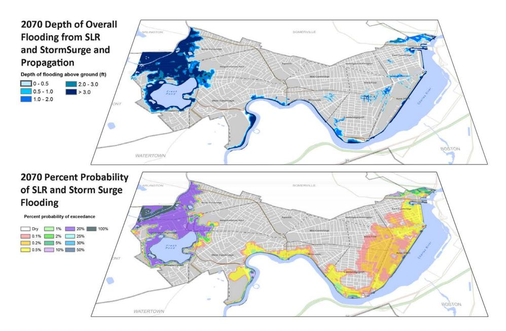
Fig. 9 Top map: 2070 Depth of Flooding from SLR and Storm Surge at 1% Probability Bottom map: 2070 Percent Probability of Sea Level Rise and Storm Surge Flooding (Source: Kleinfelder, February 2017, based on WHG MassDOT Boston Harbor Flood Risk Model)
