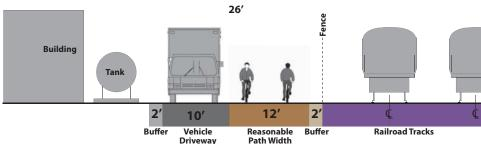
A more reasonable width for a multi-use path with a service drive that meets the constraints of this portion of the Grand Junction Corridor is 26 feet. This would be composed of a 12-foot multi-use path with a 2-foot buffer along a fence separating the rail easement. There would be no buffer between the path and the service drive and the service drive would remain at 10 feet wide with a 2-foot buffer against the buildings.
