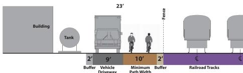
At many locations in the corridor the width falls below 26 feet to 23 or 24 feet. Rather than have the service drive overlapping the multi-use path, a narrower cross section was developed for these locations. A viable cross section can be as narrow as 23 feet and would consist of a 2-foot buffer along the rail fence, a 10-foot multi-use path, a 9-foot service drive and a 2-foot buffer.
