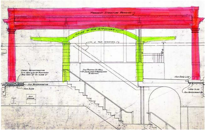
Sectional view of the new and old kiosks, looking north and showing the original staircases. Green = outline of new structure; Pink = brick structure to be removed.
