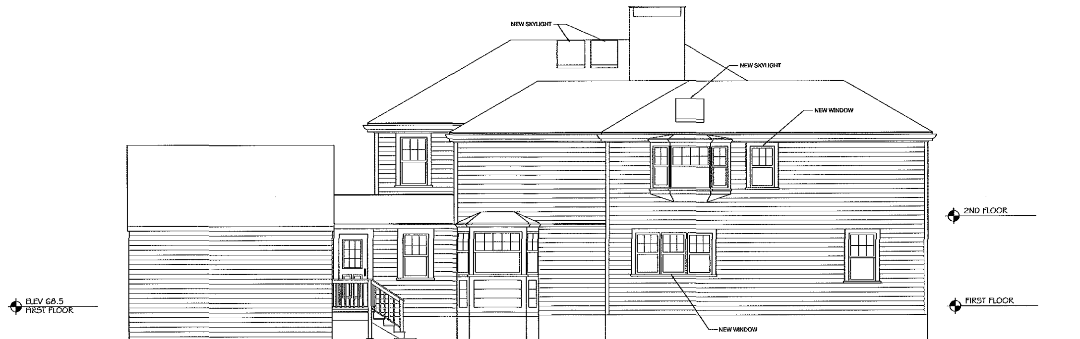
PROPOSED NORTH ELEVATION SCALE: 1/4" = 1'-0"
