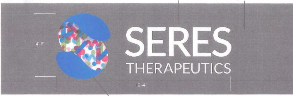
Blue sections - 3" deep fabricated aluminum Center section - 2" deep fabricated aluminum
