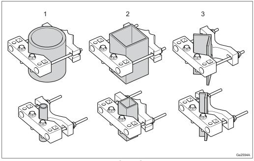
Figure 5 Alternative Pole or Mast Cross Sections
