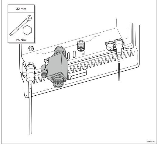
Figure 14 RF Monitoring Interface Connection
