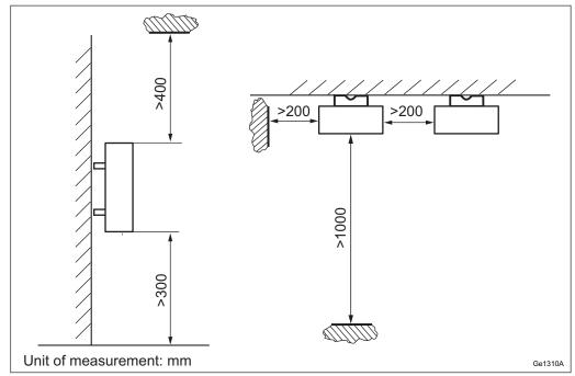
Figure 4 RRUS Wall Installation Requirements
