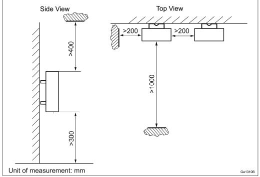
Figure 6 Space Requirements for Climate and Maintenance
