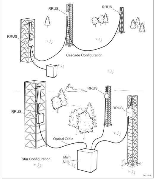
Figure 1 RRUSs in Star and Cascade Configurations
