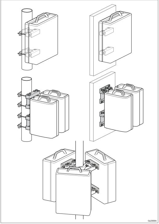
Figure 4 Installation Alternatives
