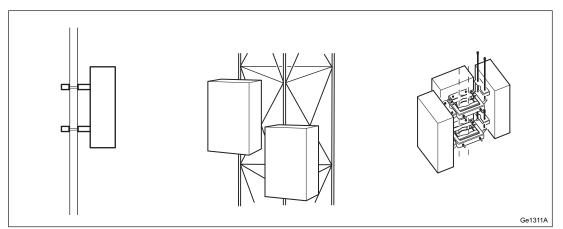
Figure 5 Sample Site Layout for Pole Installation
