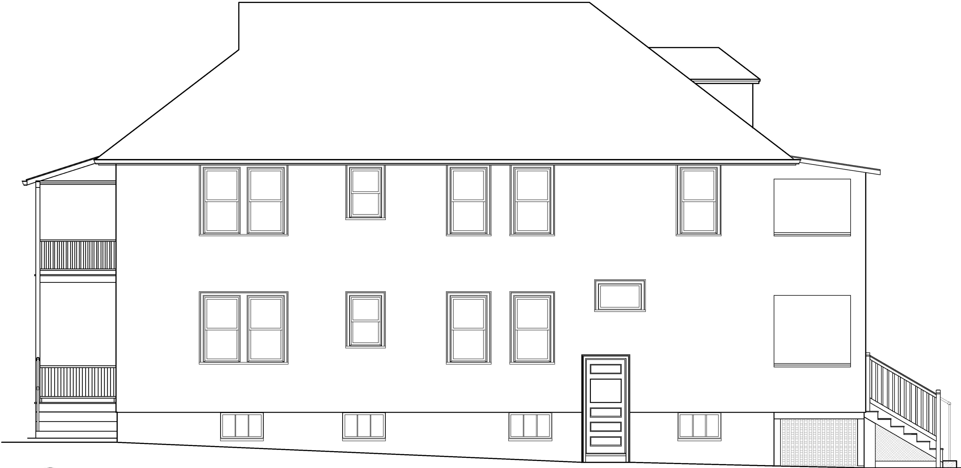
1 Existing Northeast Building Elevation Scale: 1/4" = 1'-0"
