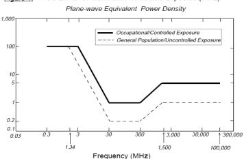
Figure 1. FCC Limits for Maximum Permissible Exposure (MPE)
