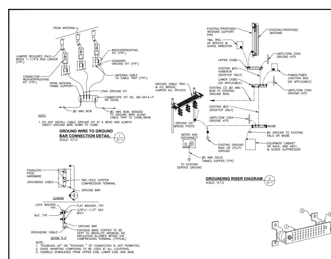
EACH GROUND CONDUCTOR TERMINATING ON ANY GROUND BAR SHALL HAVE AN IDENTIFICATION TAG ATTACHED AT EACH END THAT WILL IDENTIFY ITS ORIGIN AND DESTINATION.
