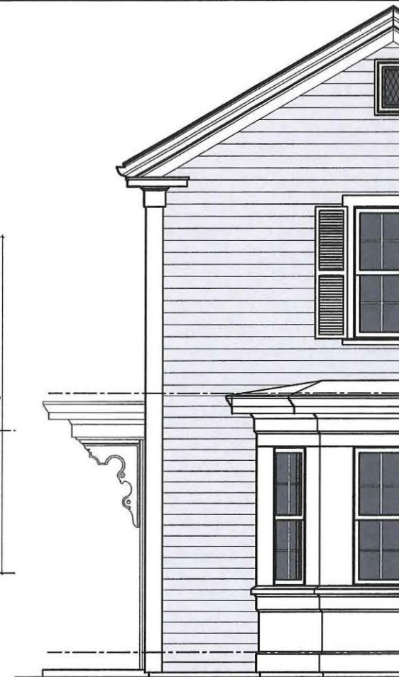
PARTIAL NORTH ELEVATION 1/2" = 1'-0"
