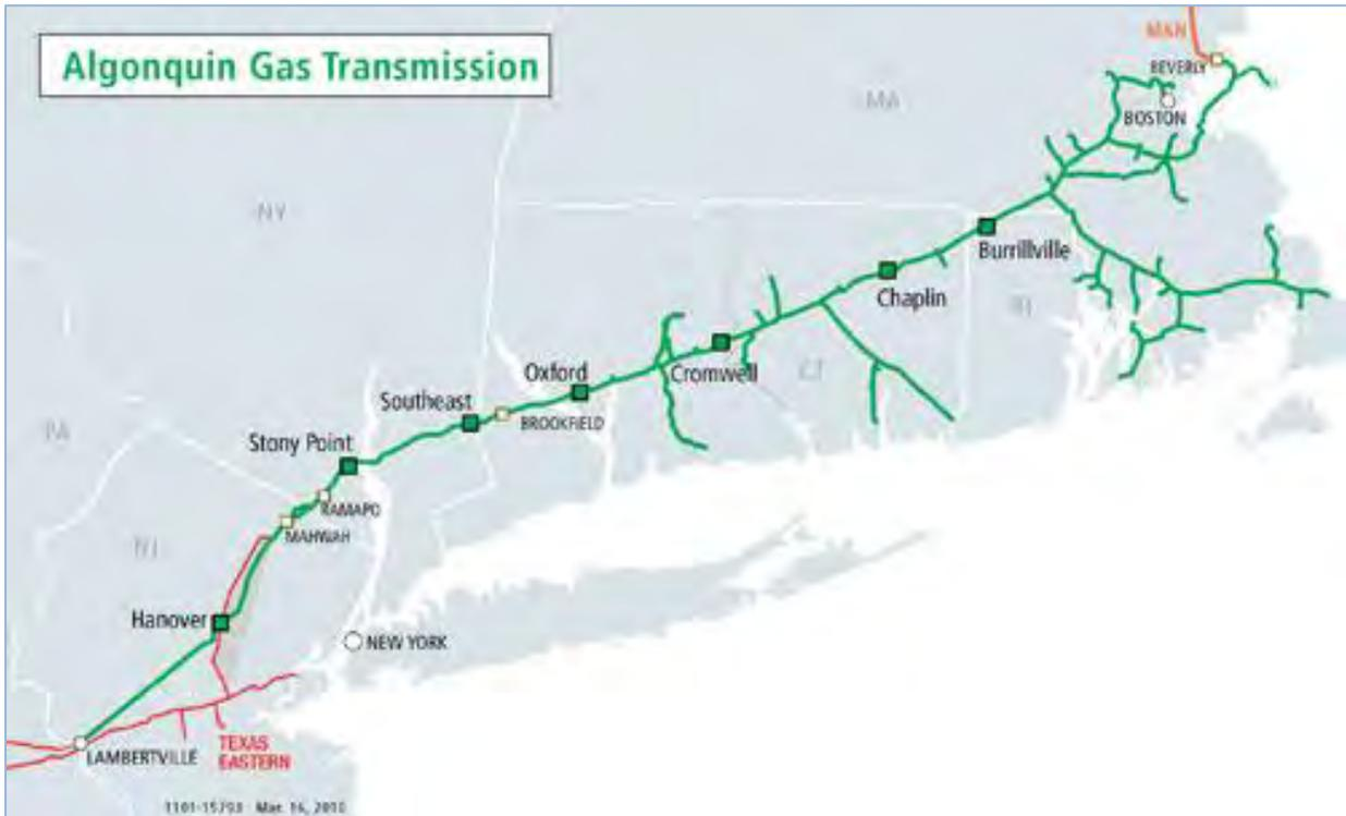
**Figure 2: Regional Diagram of Algonquin Pipeline<sup>24</sup>**
