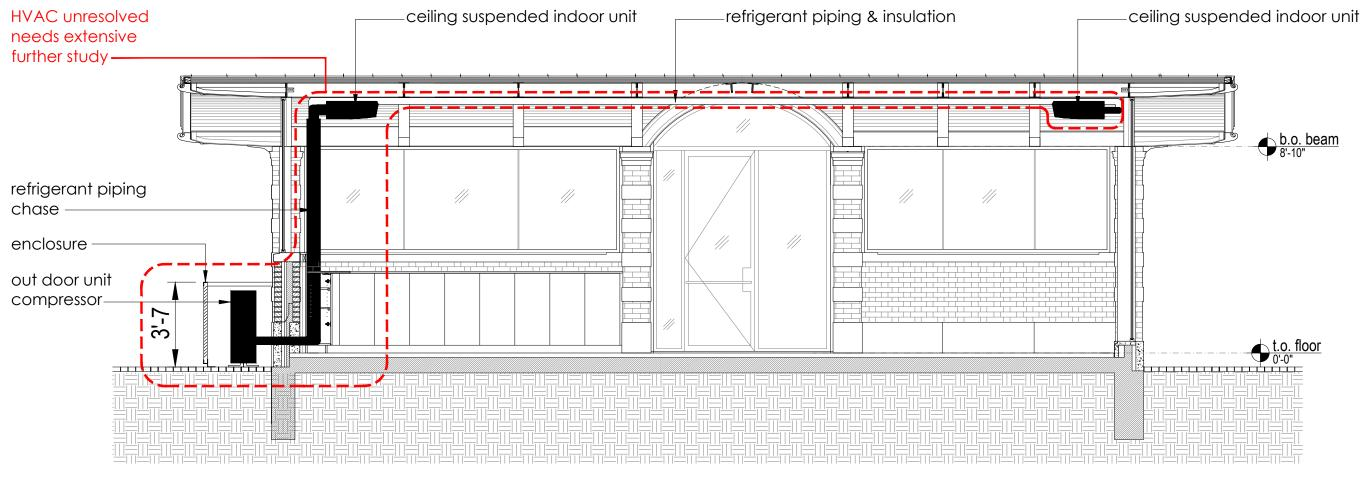
Building Section - Ceiling Suspended Heat Pump
