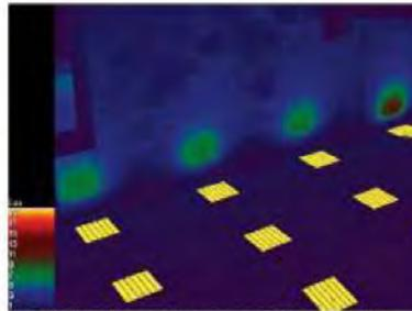
Simulation False Colour rendering showing light spill from roof lights
