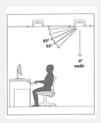
"For all regularly occupied spaces, use light fixtures with a luminance of less than 2,500 cd/m² between 45 and 90 degrees from nadir." – LEED v4
