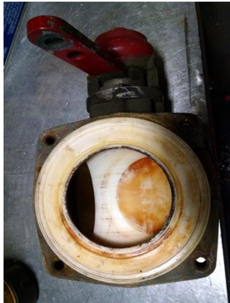
Also discovered was a drain that didn't work. After the motor squad removed the drain, they found debris had clogged the drain. If this stuff is in the drain, it's in your pump and could be plugging your nozzle!
